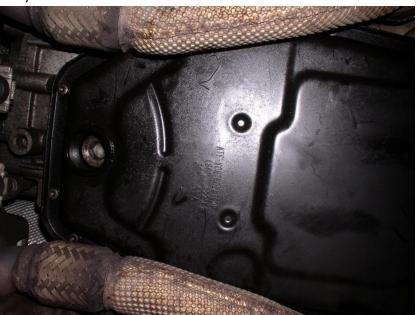
Passenger/Driver Exhaust connection to the down pipes When refitting the driver side, I used some tape on the u-joint to stabilize it just enough to guide the bolt back on the stud. It worked pretty well.:
