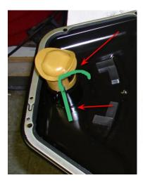
Poor attempt at drawing the path the fill tube has to take
