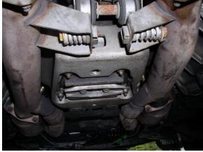
Once the front bolts, the rear couplers and the center supports have been removed the exhaust will be free. The passenger side can be lowered to the ground, but for the driver side, since I did not want to disconnect the 02 sensors, I used jack stands to support the exhaust sections that I disconnected. Driver side supported and passenger side removed:
