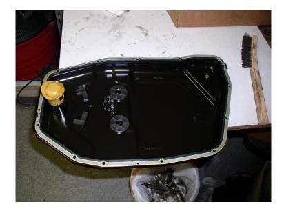
6. Remove the filter (not my filter, forgot to take a shot of it in place). There are no fasteners, just the seal holds it in place. Let the rest of the fluid drain out:
