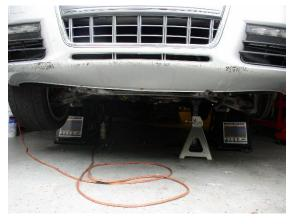
2. First thing you will see is the exhaust is in the way (I took the center sections apart, but did not have to). The passenger side was easier to deal with than the driver side (the bolts were up out of the way and required some extensions and u-joints):
