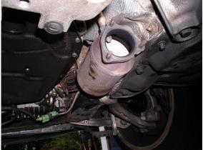
3. There are some wires and coolant hoses you will need to move out of the way by disconnecting the mounting brackets near the oil cooler. I also protected them from the oil draining out with some aluminum foil:
