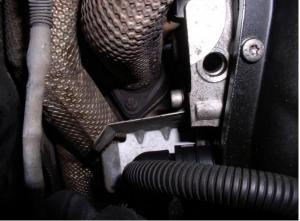
Remove these connections toward the rear as well as the support brackets in the center
